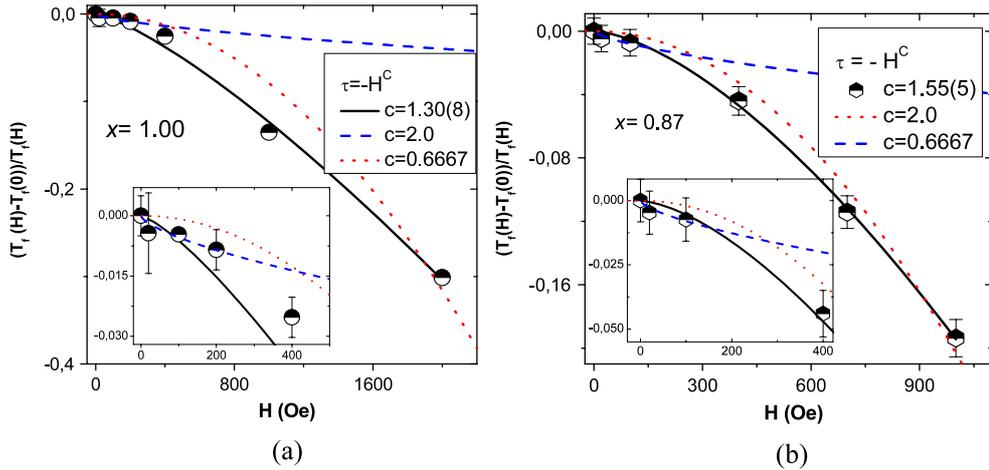
**Figure 6.**  $H-T_f$  diagrams for  $Zn_{1-x}Mn_xIn_2Se_4$  with (a)  $x = 1.00$  and (b)  $x = 0.87$ . The solid curves represent the fit of data; dashed and dotted curves represent the AT and GT lines, respectively.
