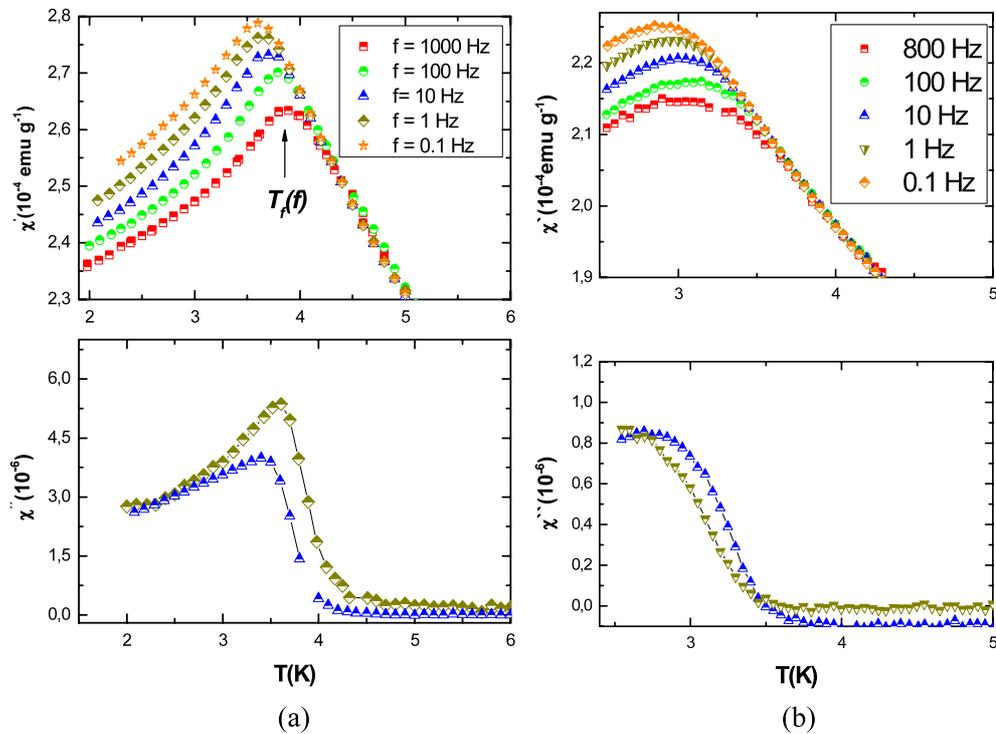
**Figure 2.** Temperature dependence of the in-phase ( $\chi'$ ) and out-of phase ( $\chi''$ ) components of the ac susceptibility measured for  $Zn_{1-x}Mn_xIn_2Se_4$  with (a)  $x = 1.0$  and (b)  $x = 0.87$ .
