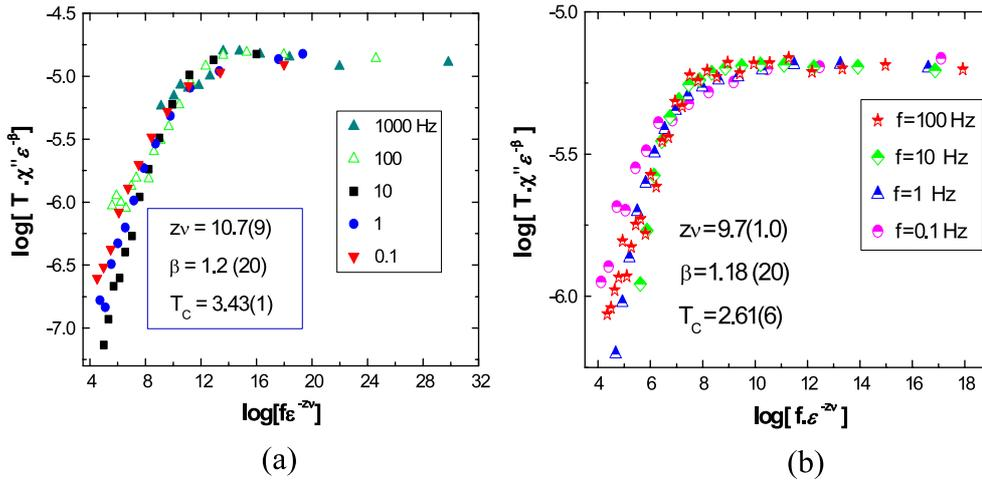
**Figure 4.** Scaling of  $\chi''(T, f)T$  performed according to equation (2) for  $\text{Zn}_{1-x}\text{Mn}_x\text{In}_2\text{Se}_4$ . (a) Corresponds to  $x = 1.00$  and (b) corresponds to  $x = 0.87$ .
