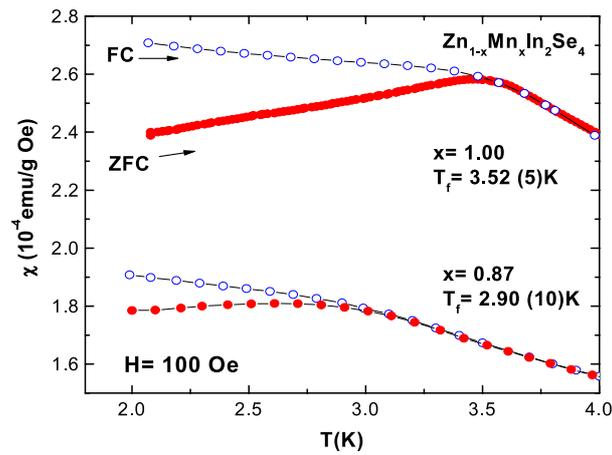
**Figure 1.** Temperature dependence of the dc zero-field cooled (ZFC) and field cooled (FC) magnetic susceptibility for  $Zn_{1-x}Mn_xIn_2Se_4$ . (Plot partially reproduced from [11].)
