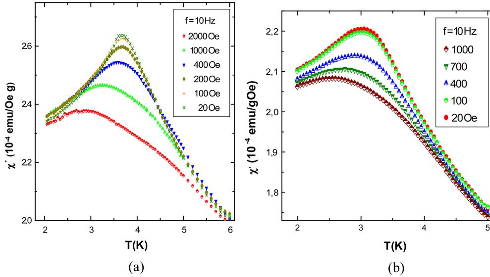
**Figure 5.** Temperature variation of the real part of the ac susceptibility obtained for different values of dc fields and  $f = 10$  Hz: (a)  $x = 1.00$  and (b)  $x = 0.87$ .
