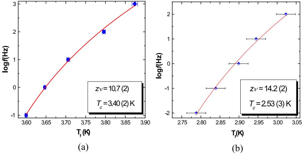
**Figure 3.** The frequency dependence of the freezing temperature  $T_f$  for  $\text{Zn}_{1-x}\text{Mn}_x\text{In}_2\text{Se}_4$  with (a)  $x = 1.00$  and (b)  $x = 0.87$ .
